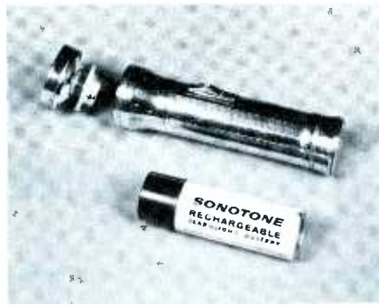
Fig. 6. Sonotone rechargeable 3-volt pack compared to 2-cell flashlight.
