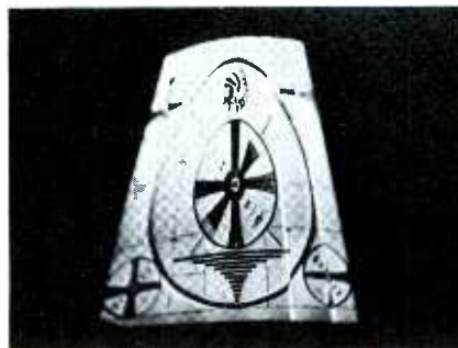
Fig. 2. When raster width is nonlinear, suspect a shorted horizontal yoke.
