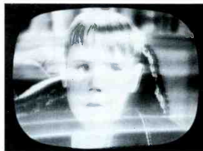
Fig. 16. Vertical-sweep distortion when video signal reaches the output grid.
