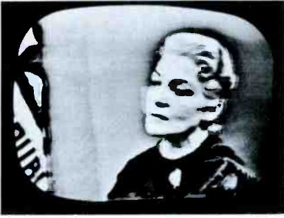
Fig. 18. Clean picture after the retrace-blanking network had been modified.
