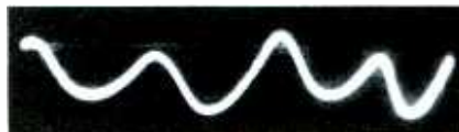
Fig. 14. Cathode signal when both B+ and bypass filters are in the same can.
