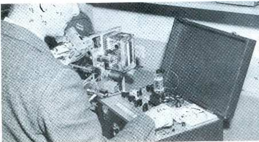
Fig. 1. Hickok's 6000 offers an automatic shorts test and quick heater check.
