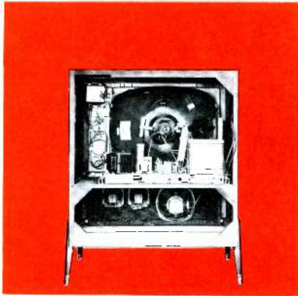
Fig. 1. Motorola Model 21K104M uses horizontally-mounted chassis with separate tuner-and-control panel.
