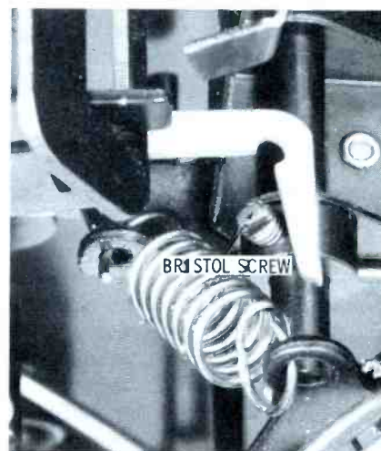
Fig. 2. Bristol set screw is used to raise lever bracket for height adjustment.
