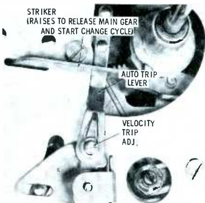
Fig. 16. Velocity-trip adjustment is beneath turntable for Garrard unit.
