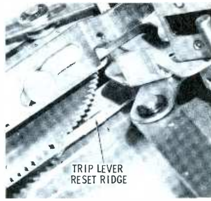
Fig. 21. Reset ridge returns trip lever to position after trip cycle has started.
