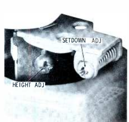
Fig. 10. Height and set-down adjustments are made with Phillips driver.
