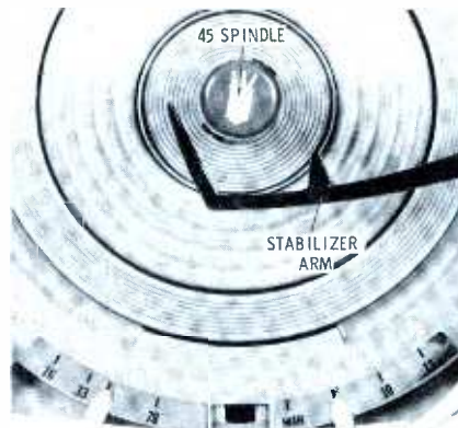
Fig. 9. Zenith crest points toward front for correct 45-rpm spindle installation.
