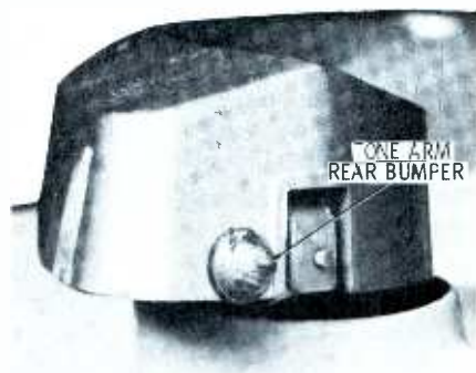
Fig. 23. Rubber bumper on tone arm.
