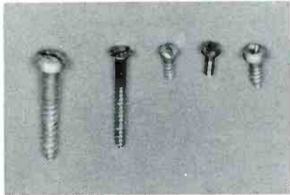
Fig. 7. Examples of "chewed-up" heads.
