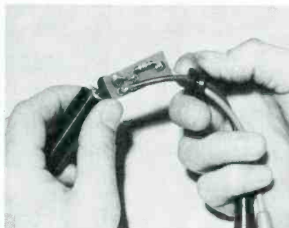
Fig. 3. Special scope-input cable with low-pass filter network termination.
