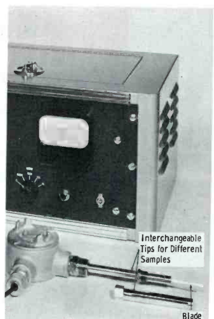
Fig. 4. Dynamic viscosity is determined from the amount of power required to make the probe blade oscillate.
