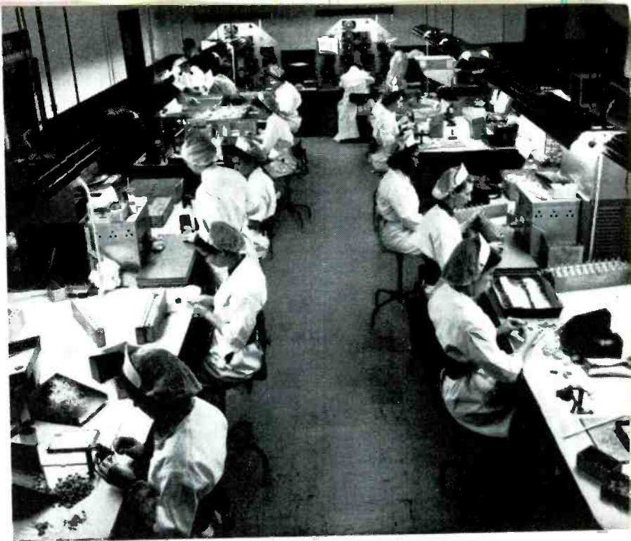
SEPARATE FACILITIES are maintained for the exclusive processing and manufacture of high reliability capacitors. Only specially trained, highly skilled operators, who wear special clothing to prevent any possible source contamination, work here.
