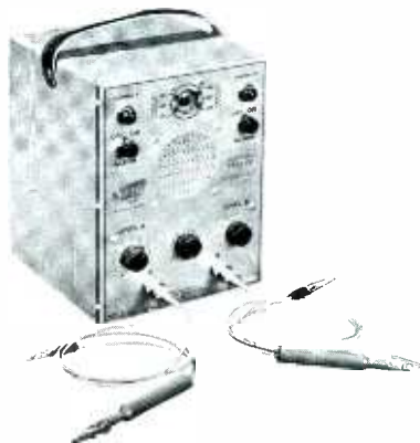
Fig. 1. Seco Model SL-10 Monitor—A Signal Tracer and Intermittent Localizer.
