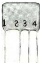
Fig. 3. Universal Ceramic Unit Capable of Providing Various Capacitances.
