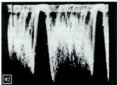
Fig. 4. Waveform Observed at Grid of V10A at 7,875 CPS and Showing Flattened Pulses Caused by Overloading of Video Amplifier.
