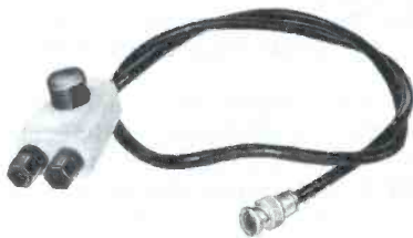
Fig. 6. Output Cable With Vernier Attenuator for the GE Sweep Generator, Type ST-4A.
