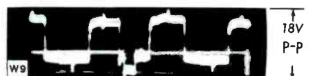
Fig. 6. Waveform W9 Indicating Abnormal Condition Ahead of the Grid of the Red Gun, As Discussed in Case History No. 2.
