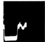
Fig. 13. Signal at Plate of the I-Demodulator Illustrating Improper Cancellation of the I Signal.
