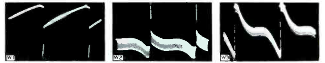
Fig. 14. Picture Display and Waveforms Resulting From a Heater-to-Cathode Short in the Vertical-Output Tube.
