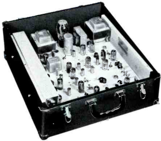
Fig. 1. Hickok 655XC Color-Bar Generator.
