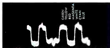
Fig. 20. Signal at Grid of Green Gun.
