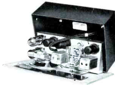
Fig. 8. The Flush Wall Radio Hinged Down for Tube Replacement.
