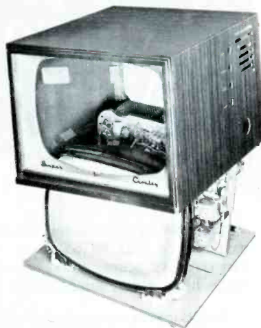
Fig. 2. The Crosley Model G-17TOMH With the Cabinet Partially Removed.
