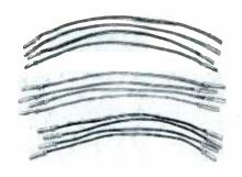
Fig. 8. Jumper Leads for Use When Working on Combinations.
