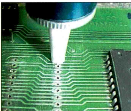
Figure 10. Once the solder has been melted, place the desoldering tool tip over the joint at an angle (trying not to touch the soldering iron's tip), then move the soldering iron away, and quickly position the vacuum tool perpendicular to the board, and quickly press the trigger. This should suck the molten solder from the joint.
