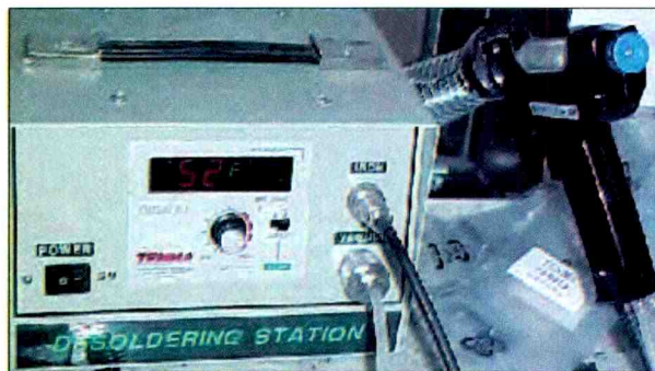
Figure 3. A more sophisticated solder station provides good temperature control, and includes a vacuum pump to speed desoldering.
