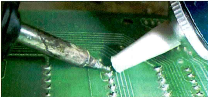
Figure 9. In order to remove the solder from a soldered connection, first heat up the solder joint with the soldering iron.
