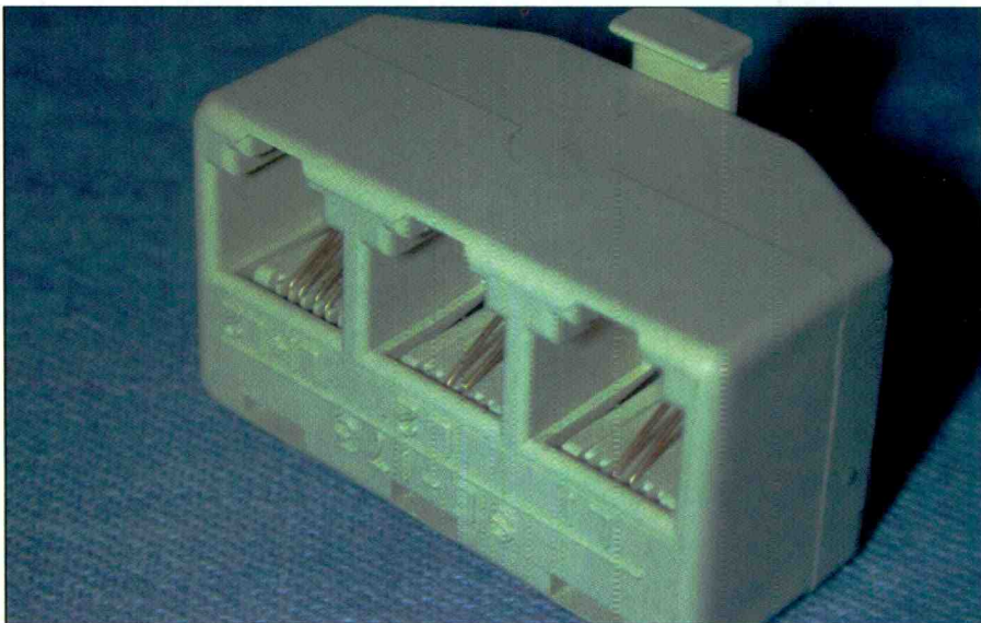
Figure 6. You can run all four wires to a modular jack, and then split out the two lines using a splitter such as this. Note that in one outlet of the splitter, the two wires of line one appear, while the two wires of line two appear at the other outlet. In this three-way splitter, both lines appear in the third outlet, so the two lines may be run further.
