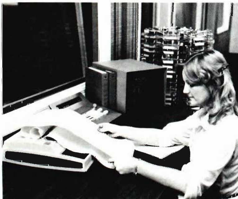
Automatic logging printout tells Cindy Hottell not only what events played at what time, but also what was scheduled to play and didn't. Logging descriptions are a full 80 character line printed in English.
