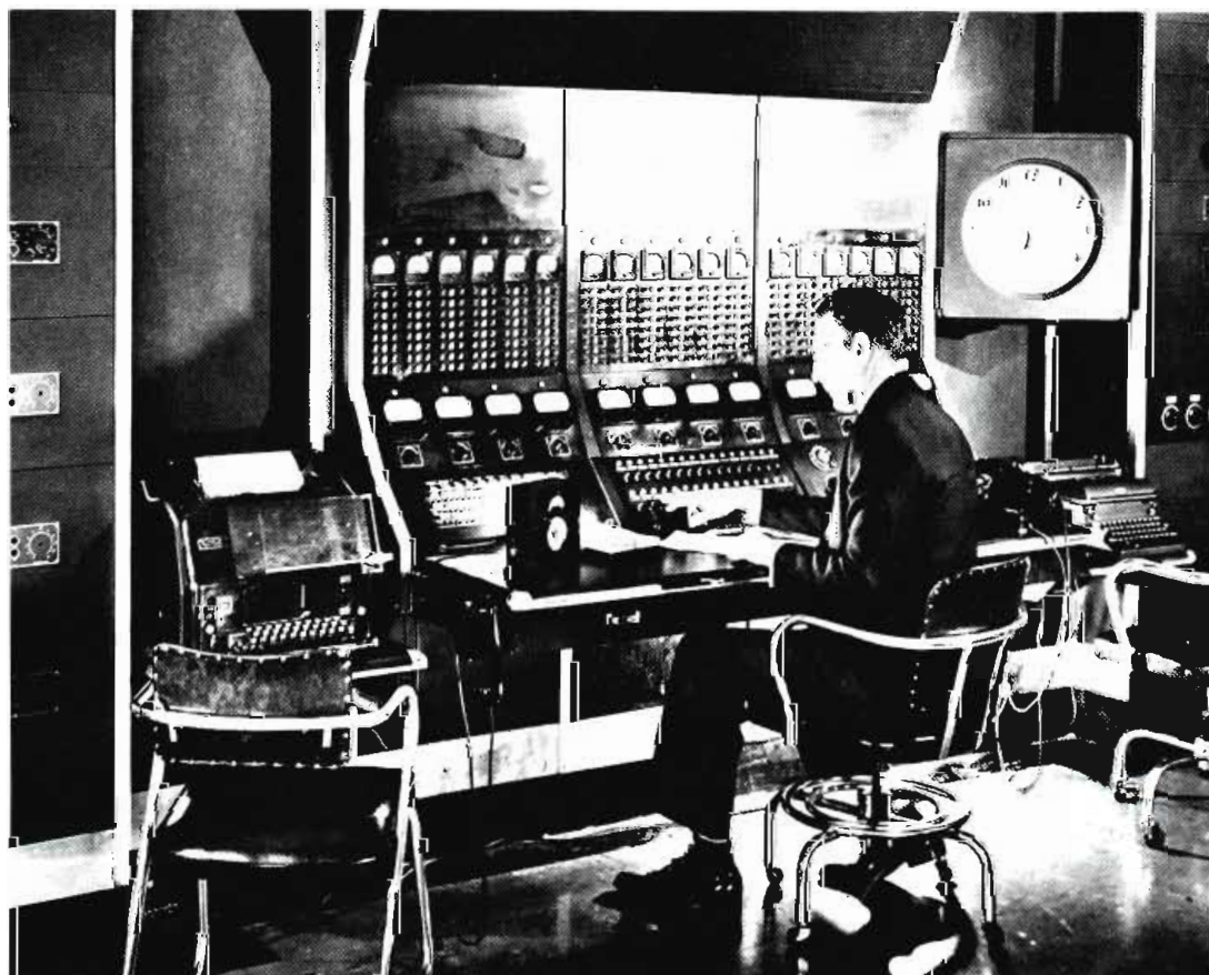
Master Control — This control center fed programming down a bank of phone lines to the transmitter site. During 500 kw years, WLW program listings appeared in up to seventy-six newspapers from Texas to Connecticut. Programs were routed to WLW, WSAI, W8XAL, the "New York Line" and various national networks.
