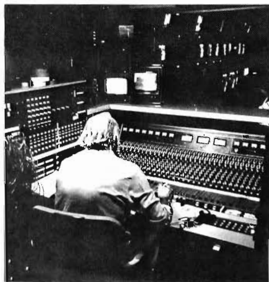
Audio engineer Scott Schachter is responsible for riding levels on upwards of 60 different mikes. A Neve 36-channel broadcast audio console is used.
