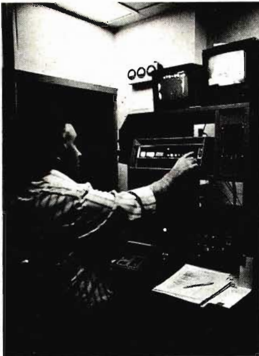
Arvin-Echo Frame Storer Model EFS-1 is used almost like a slide projector. A still frame is stored by Mike Madigan to be used later with sketch credits.
