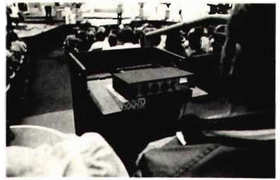
Engineer controls in-studio PA with a Shure M63 Audio Master mixer. Microphones used on program are generally Sony ECM 51 condenser units.
