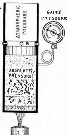
FIG. 16.—Elementary boiler or closed vessel illustrating the difference between gauge , and absolute pressure .
