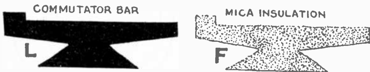
FIGS. 605 and 606.—Mica segment F, cut from sheet using bar L, as pattern. Such a segment is cut large at top and at ends so as to turn down evenly with copper bars when commutator is finally surfaced. Clamping toes and foot must be thinned to allow for give of copper bars and to obtain tight clamping of mica on the outside of commutator. Make toes .003 to .004 ins. thinner; lower edge .002 thinner.
