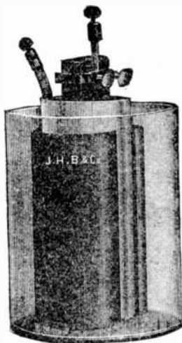
FIG. 154.—Bunsen cell. This is a two fluid cell and has a bar of carbon immersed in strong nitric acid contained in a porous cup. This cup is then placed in another vessel, containing dilute sulphuric acid, and immersed in the same liquid is a hollow cylindrical plate of zinc, which nearly surrounds the porous cup. The hydrogen starting at the zinc, traverses by composition and recombination, the sulphuric acid; it then passes through the porous partition, and enters into chemical action with the nitric acid, so that none of it reaches the carbon. Water is produced by this action, which in time dilutes the acid, and orange colored poisonous fumes of nitric oxide rise from the battery. If the nitric acid first be saturated with nitrate of ammonia, the acid will last longer and the fumes be prevented. Strong sulphuric acid cannot be used in any battery; one part of sulphuric acid is generally added to 12 parts by weight, or 20 by volume, of water. Grove used a strip of platinum instead of carbon in his cell. A solution of bichromate of potassium is frequently substituted for the nitric acid in the porous cup, thereby avoiding disagreeable fumes. Bunsen's and Grove's cells produce powerful and constant currents, and are well adapted for experiments, but they require frequent attention, and are expensive, so that they are little used for work of long duration. The electromotive force of these cells is about 1.8 volts.
