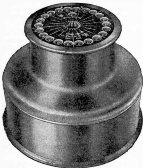
FIG. 679.—Chapman style C armature. It indicates the condition of all parts of a wound armature simultaneously; will test the armatures it was built for as specified, will also indicate shorts in double voltage and open circuits on half voltage windings at equal speed. The operator cannot ignore defects. The indications stand out and command attention. A pilot lamp is provided to show the correct reading of the indicators. To operate , the commutator is inserted in the center of the top whereupon the indicators will light up half way if everything be O.K.; if not, there will be an irregularity in their illumination. This irregularity is what the operator looks for. If a bare commutator be tested, no response is made by the indicator unless a short or ground be present. The odd indicator is assigned to reading grounds at the working voltage of the armature.
