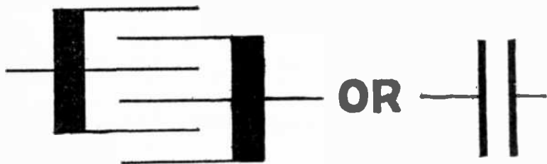
FIGS. 344 and 345.—Conventional diagram of a condenser. A condenser is a device designed to absorb or hold an electric charge in about the same manner as a vessel will hold a liquid. Every conductor of electricity forms a condenser and its capacity for holding a charge depends upon the extent of its surface. A condenser is therefore made of conductive material formed into such shape as to present the maximum surface for a given amount of material.
