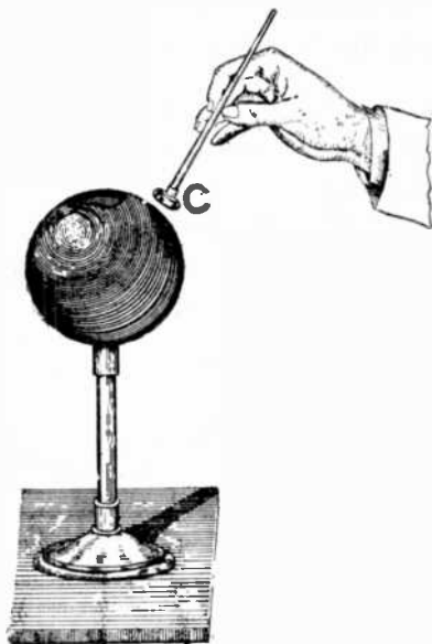
FIG. 49.—Distribution of electrification on a charged hollow sphere. If an insulated conductor C, be inserted through the opening in the sphere and brought into contact with the interior surface and afterwards carefully removed, it will be found, by testing with the gold leaf electroscope, that it has received no charge. If touched to the outside, however, the conductor will receive part of the charge.
