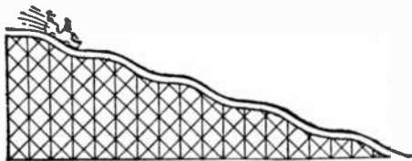
FIG. 420.—Direct current fluctuations. The current in the circuit fed from a dynamo fluctuates continually in value, but with a large number of commutator segments the magnitude of these fluctuations is entirely negligible. The disturbance that might be produced by such fluctuations may be compared to the changes in speed that would be produced in a car by waves in the track of an inclined railway; that is, a few large waves would produce greater disturbances than a large number of small waves. Likewise a large diameter commutator will produce a steadier current, and consequently a steadier light than a small commutator with a smaller number of segments.
