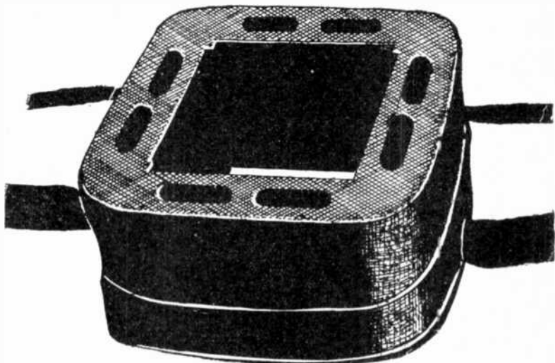
FIG. 534.—Compound wound rectangular ventilated spool field coil. The series and shunt coils are wound side by side, ventilating passages being provided lengthwise through each coil and between the shunt and series coils as shown.
