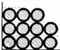
FIGS. 527 and 528.—Square and hexagonal order of "bedding." The term bedding is an expression used to indicate the relation between the cross sectional area of the winding when wound square, as in fig. 527, and where wound in some other way, as in fig. 528. In the square order of bedding, the degree of bedding equals zero.
