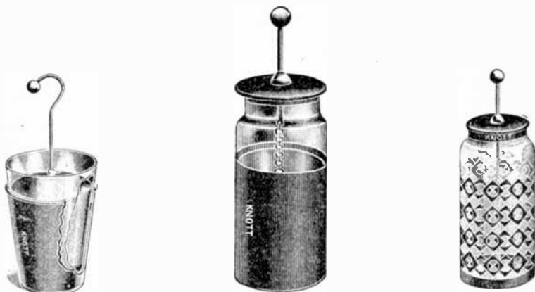
FIGS. 75 to 77.—Knott demonstration Leyden jars for demonstrating that an electric charge resides as potential energy in the glass of a Leyden jar and not in the metallic coatings. This is a dissectible Leyden Jar, the outer metallic covering being removable as well as the inner. The inner is provided with a rod with ball terminal for charging.
