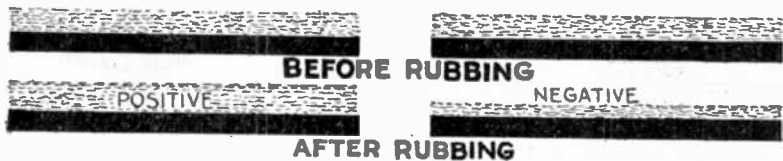
FIGS. 19 to 22.—Positive and negative electricity. The rubbing process removes electricity from one body transferring it to the other.
