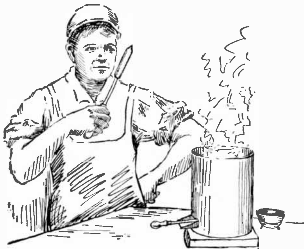
FIG. 217.—Method of judging the heat of a soldering bit or so called "iron," illustrating sensible heat .
