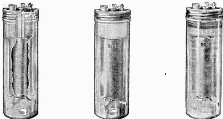
FIG. 146.—Waterbury telecell zinc cylinder cut away to expose the interior construction of the cell to inspection. The perforated cylindrical basket inside of the zinc cylinder contains the depolarizing element, that is, copper oxide. The small legs and feet at the bottom keep elements centralized. The copper oxide is sealed in the basket to prevent sifting out during shipment.
