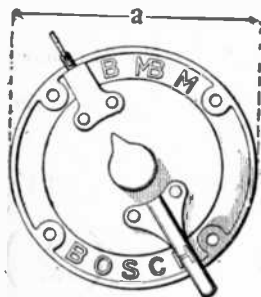
FIGS. 370 and 371.—Bosch type C horizontal secondary coil. The parts are: 1, switch handle; 2, movable cover; 3, coil housing; 4, starting press button; 6, fixed connection plate; 7, movable switch plate; 8, cable cover; 9, milled edge nut; 10, iron core; 11, plate carrying the starting arrangement and the condenser; 12, condenser; 13, contact spring; 14, vibrator; 15-16, auxiliary contact breaker; 17, vibrator spring; 18, stop screw for switch handle; 24, locking key.
