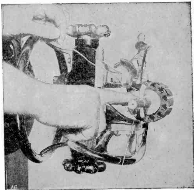
FIG. 656.— Chapman moving picture 2. When the proper number of turns are on, place the finger on the head of the armature; over the first lead. Pull it off the snubbing pin, it will come easily. Pull it down to the left, and slightly upward as shown.
