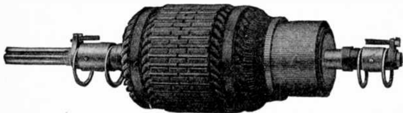
FIG. 581.—Fairbanks Morse type TR machine armature constructor. The armature core, is built up of thin sheet steel laminations with notches in the circumference, which, when the discs are placed together, form grooves or slots to receive the armature coils. With specially designed tools these notches are so accurately spaced that no filing of the slots is required. The armature cores for the Nos. 23, 24, 25, 26, 27, 28 and 29, machines are mounted on a cast iron spider, which also carries the commutator, making the two parts entirely self-contained, and with this construction, it is possible to remove the armature shaft, without disturbing the core, commutator or windings.
