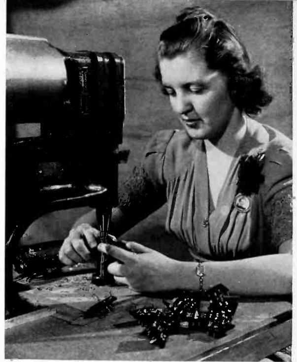
"Squeeze riveting" is an important operation in the manufacture of radio parts for Signal Corps equipment. The "Riveter" wears her identification badge
