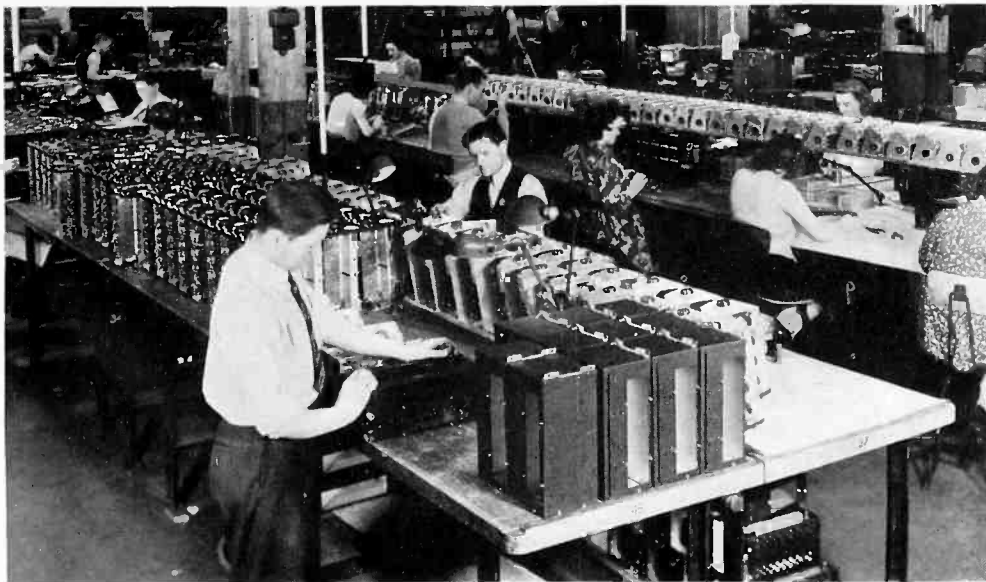
Rows of radio receivers for the Air Corps are being wired by these expert craftsmen
