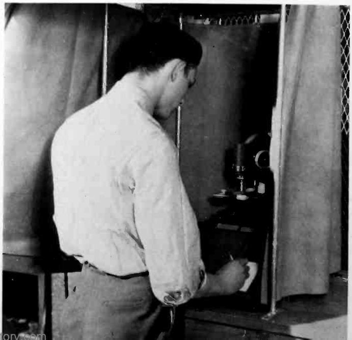
Small parts from outside firms go through rigorous micro-projector tests before they are incorporated in assemblies
