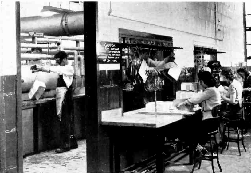
Before getting their enamel coatings these housings pass through dipping and shielding operations. Equipment will be installed on fighter planes.
