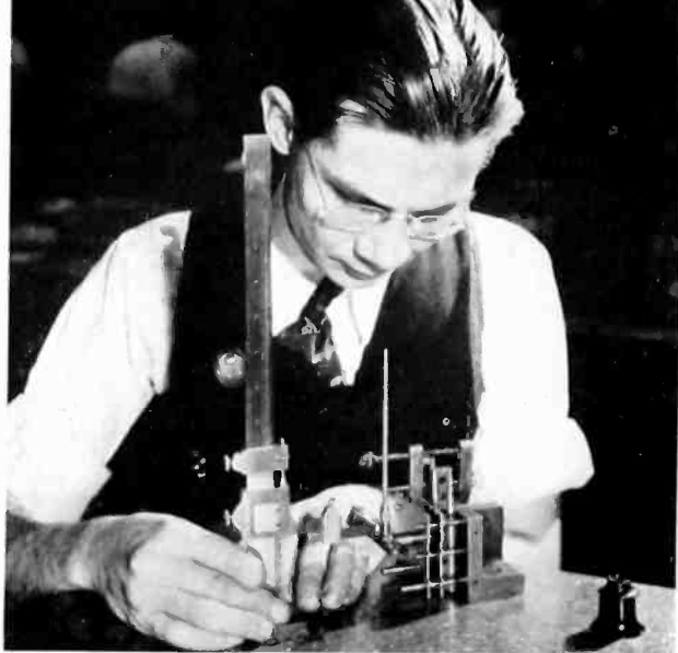
Height gauge and dial indicator implement the checking of radio parts to a tolerance within .0005 of an inch
