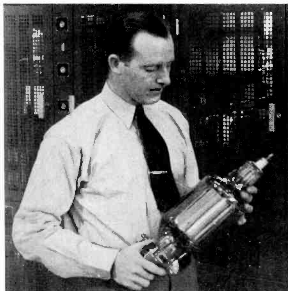
Walter W. McCoy, chief engineer of station WJAS, Pittsburgh, Pennsylvania, holds a 279A vacuum tube which was removed from the station's transmitter after 16,297 hours of operation. Although still functioning it was removed at the end of this period because the station feared it might fail and cause lost time on the air.
