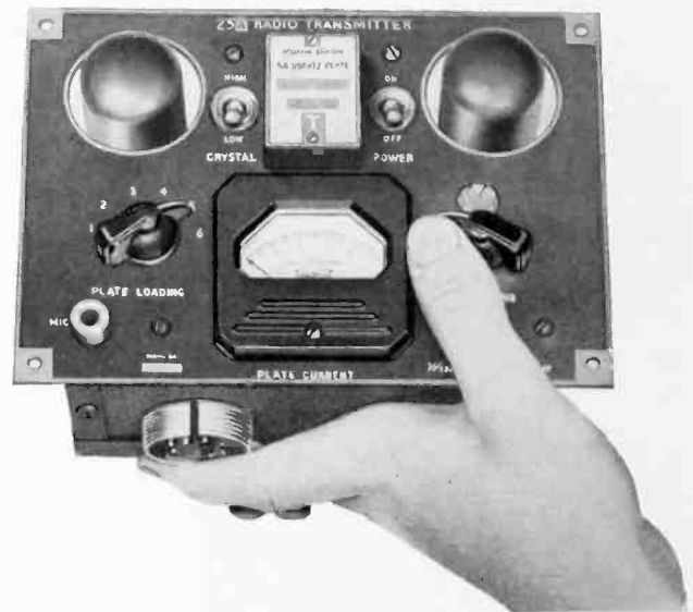
The Western Electric 25A multi-frequency radio transmitter specially designed for installation in private planes.
