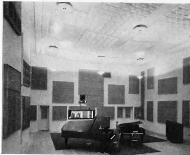
Figure 1. One of World Broadcasting's new studios in Chicago in which the many acoustic surfaces are plainly seen. Photograph made before any form of decoration was applied.
