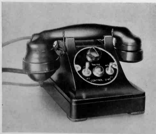
The standard handset on which are located all of the controls necessary for the remote operation of the equipment.
