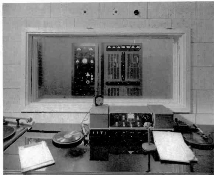
Below: The 310B Transmitter (seen through wall panel) 23A Speech Input equipment, salt shaker mike on desk.
