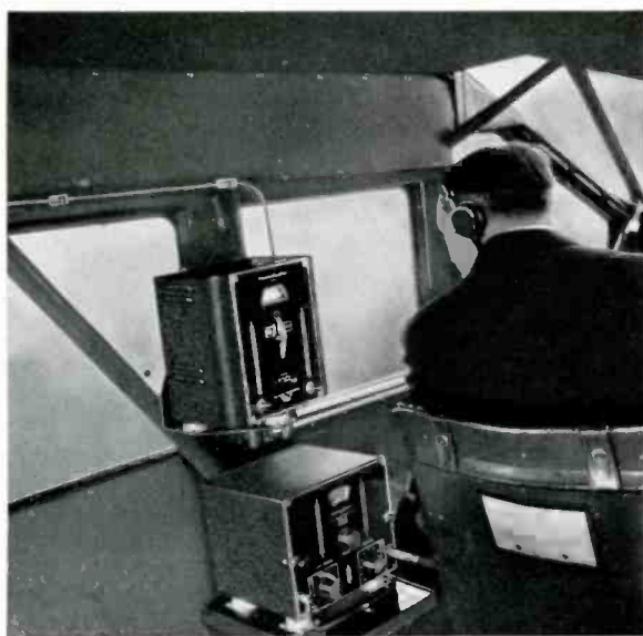
The 19A Midget Transmitter and the 17A Receiver installed in a plane — a complete two-way system.
