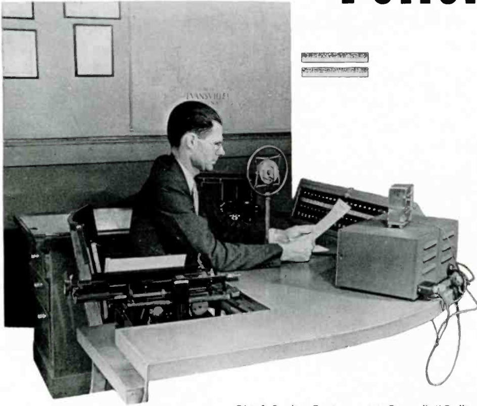
Chief Radio Engineer McConnell "Calling All Cars." At his left, P Receiver—at right, an amplifier—in the center, a signal board contain of red lights at top and green lights at bottom with car numbers in be
