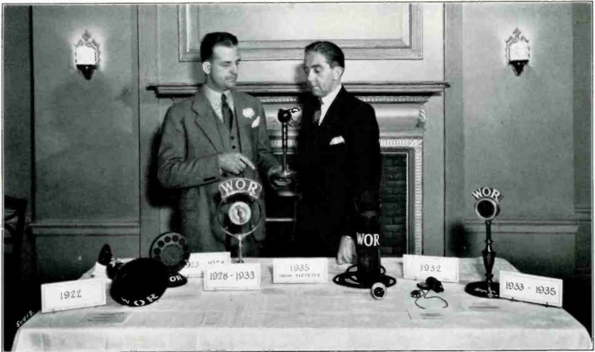
J. R. Poppele, WOR'S chief engineer, showing Alfred J. McCosker, president of the Bamberger Broadcasting System, Western Electric's new non-directional dynamic microphone. Displayed on the table is the evolution of microphones used at WOR since the inception of the station: (left to right) telephone transmitter with megaphone (1922); double carbon button (1923-28); improved double carbon button type with improved mounting (1928-33); condenser microphone with amplifier (1928-33); lapel microphone (1932); dynamic microphone (1933-35).
