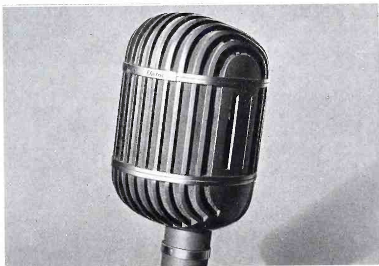
tions of infant art of telephony. The box telephone is thus the grand-daddy of all modern microphones, represented by the Western Electric Cardioid, right.
