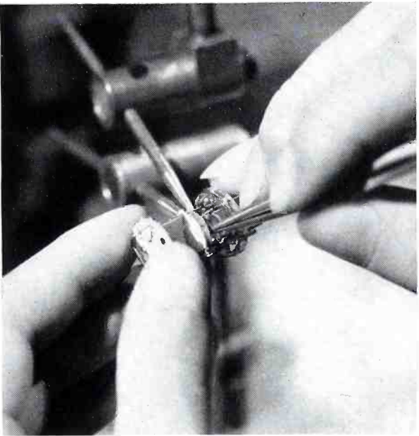
10 Spotwelding fastens structure together securely and joins it to leads in glass stem. This close mounting is important at higher frequencies.
