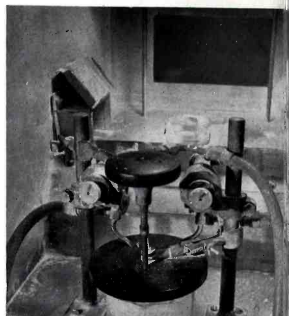
2 Here the cathode elements, mounted in the circular jig, pass before spray guns which coat them uniformly with a triple carbonate mixture.
