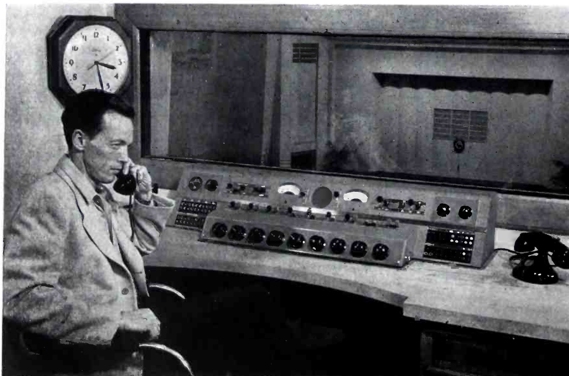
Below: Rex Morrow, assistant chief engineer, seated at the 40A Console section of the Western Electric 25B Speech Input Equipment. Studio B, which seats 450 people, can be seen through control room window.
