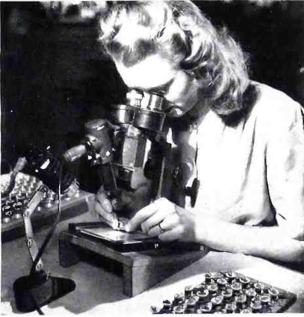
11 Finished mount structures receive a critical inspection under a microscope, then are tested for "shorts" and "opens" before proceeding to next step.
