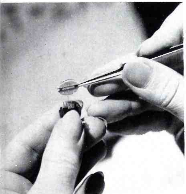
9 Next, the top mica and getter are placed in position. Although the individual parts are fragile, finished structure is extremely rugged.
