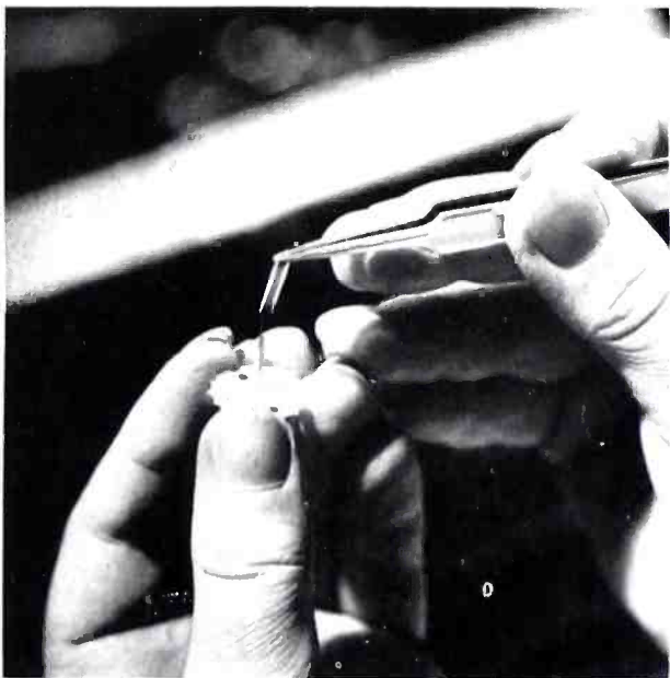
6 Next come the grids. Here the first is put in position. Care must be taken not to damage the extra fine wire, which may be only .001 inch in diameter.
