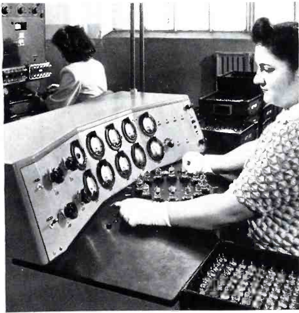
16 Each tube receives a thorough electrical test. Console-type test equipment is shown in foreground; rack-mounted type is shown in upper left.
