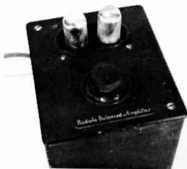
Radiola balanced amplifier was a desirable accessory for the Radiola III, enabling the little set to drive a loudspeaker.
