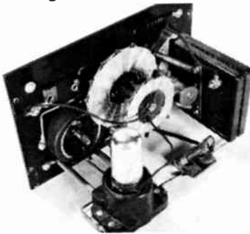
"Regen" sets squeezed amazing performance out of one tube. Note pancake coils in feedback circuitry of Crosley 50. Rear one is adjustable.
