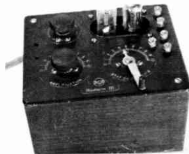
RCA Radiola III was more elegantly made than the Crosley 50 and boasted an additional tube that provided extra headphone volume.
