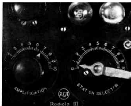
Besides rheostat(s) for filament voltage, regenerative sets generally required only regeneration ("amplification") and tuning controls
