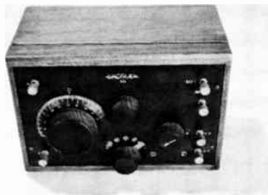
Crosley 50 was probably the most widely sold single-tube regenerative receiver of the early 1920's.
