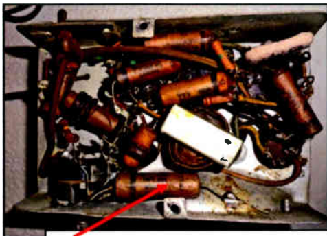
If this .05 mfd capacitor fails as a short, the chassis and floating ground are common—a shock hazard!
