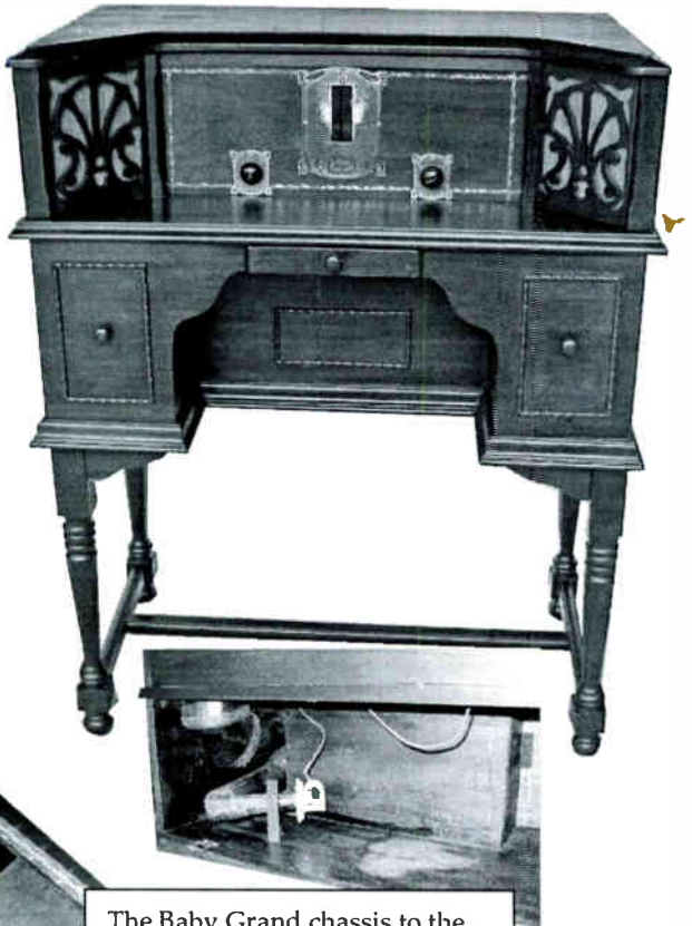
The Baby Grand chassis to the left and the battery box above. Note the battery acid damage. The damage is visible under the box as well.
