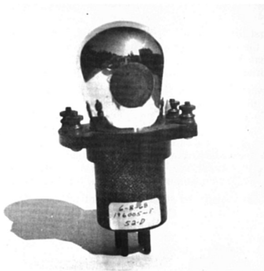
Fig. 1 The Van-Horne/Musselman triple was the first U.S. multiple-section radio tube.
