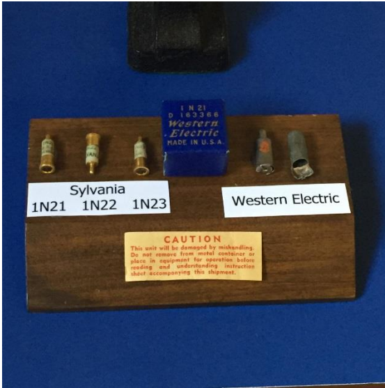
Sylvania and Western Electric crystal diodes used for radar work during World War II
