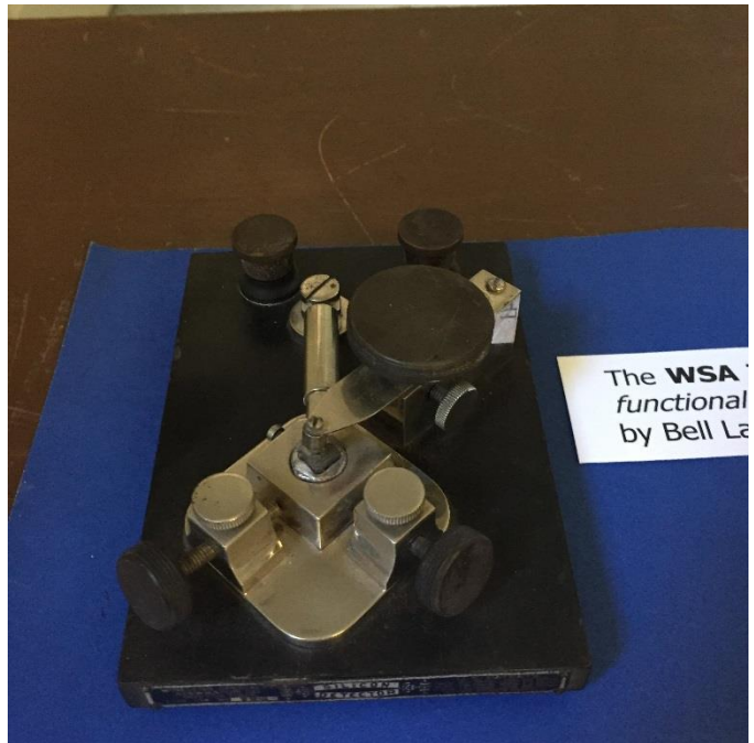
Wireless Specialty Apparatus IP-200 silicon detector, ca. 1919, Dick Howard
