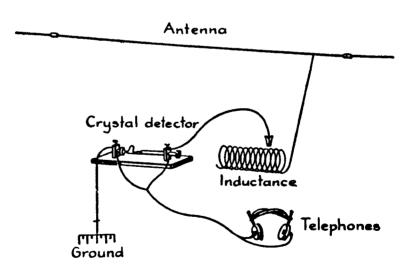
The essentials of receiving radio signals, comprising the antenna, inductance coil for tuning, crystal detector, telephones, and the ground.
