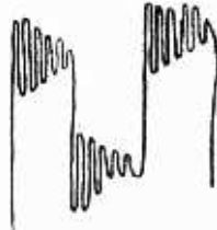
Fig. 6. Square-wave response of an amplifier showing high frequency oscillation.
