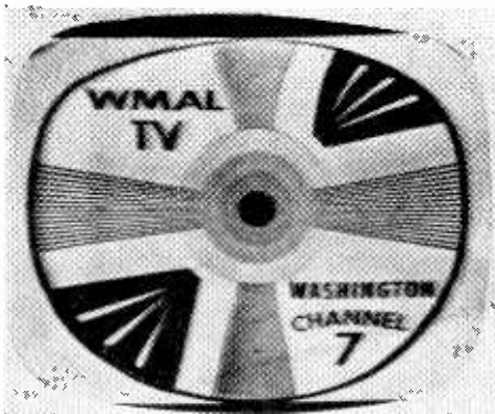
FIG. 12. Short Picture resulting from Insufficient Vertical Height.
