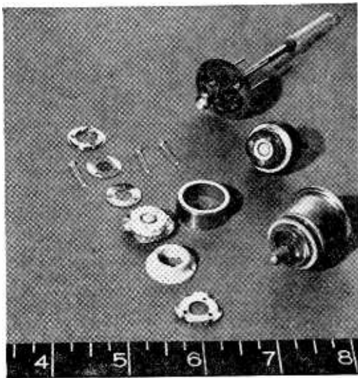
Here are the elements of the close-spaced microwave triode. The upper and lower items at the right are the tube base holding the heater leads and the tube envelope; the rest are components. The inch scale indicates the small size of the tube.
