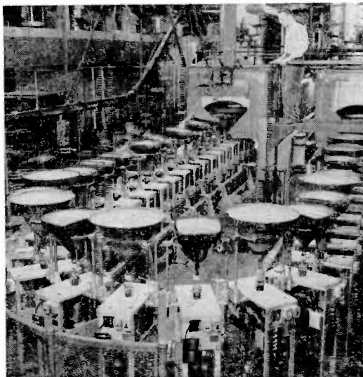
A very large in-line exhaust machine. Each "buggy" has an oil diffusion pump which creates a vacuum. Tubes go through a bake-out process in the tunnel at 400 degrees centigrade.
