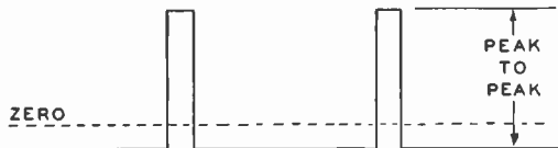
Fig. 5. Illustration of what is meant by the peak-to-peak amplitude of a pulse signal.
