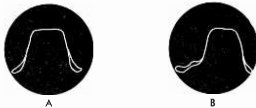
Fig. 15. (A) Typical i-f response curve for a receiver with "intercarrier" sound; (B) typical i-f response curve for receivers having a separate sound channel.
