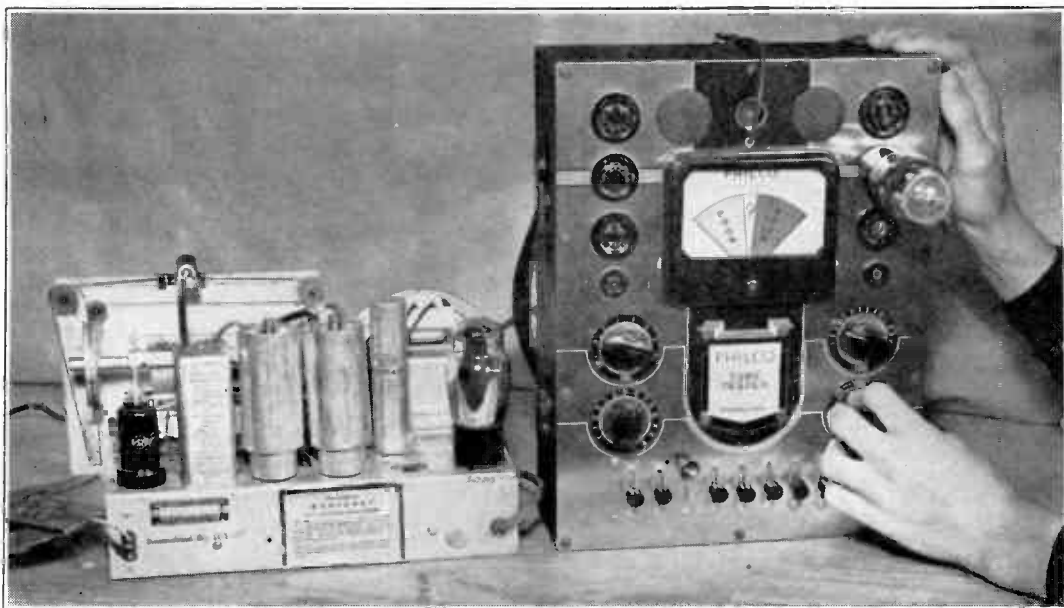
Fig. 2—Even without a cover or a carrying compartment for the line cord, this Philco Model 050 is working out nicely as a portable tube tester for either bench or home use. Here's a tip—when testing tubes, take out only one at a time as
