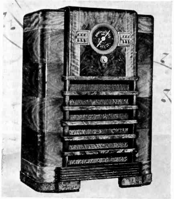
The Stewart-Warner model A-6 A.C.-D.C. superheterodyne comes in a choice of either ivory or walnut moulded plastic cabinets. Tuning and volume are controlled by the drum dials at each end of the cabinet.
