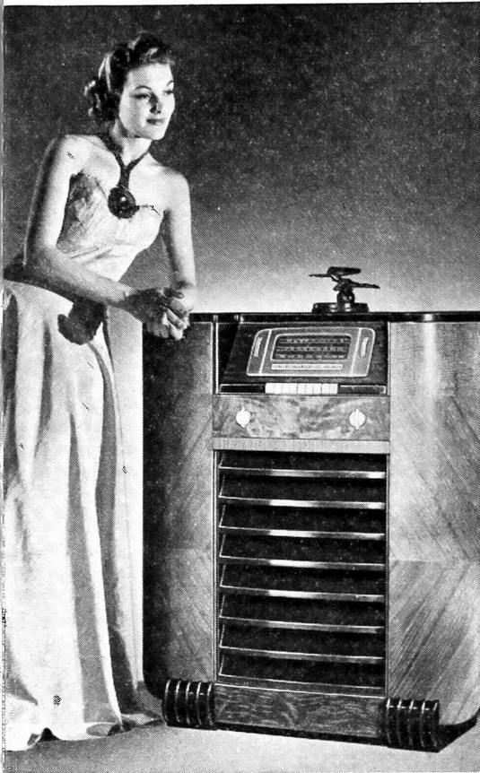
The General Electric model H-116 is an 11-tube three-band receiver. Some of its features are: the beam-oscope; Television sound or phonograph connections; automatic tuning for eight stations, automatic tone compensation and a cathode-ray tuning indicator. Iron-core coils are used in the I.F. transformers and automatic tuning circuits to eliminate frequency drift.
