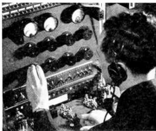
A "circuit patrolman" behind the scenes, monitoring a Radiotelephone connection without interrupting the conversation.
