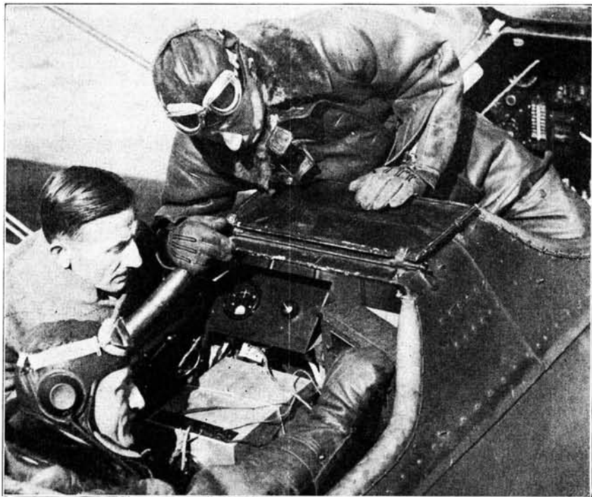
Army Air pilots making tests with plane equipped with Kruesi Radio Direction Finder. Device permits pilot lost in fog to tune in any Radio station, regardless of the program, and direct himself to that point. The inventor, G. G. Kruesi, of Transcontinental-Western Air Inc., is shown at bottom of picture.
