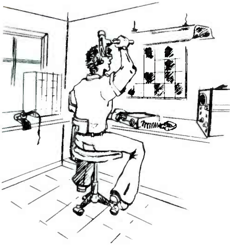
TAPPING THE P.C. BOARD TO LOCATE SENSITIVE AREA.
