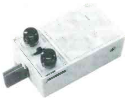
FIGURE 2. COS/MOS KEYER BUILT INTO TRANSISTOR RADIO CASE.
