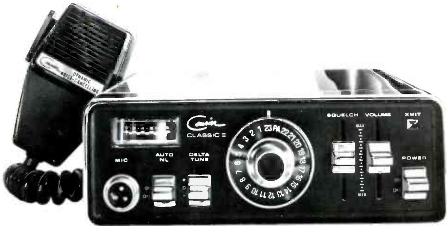
FIGURE 1. COURIER "CLASSIC II" 23-CHANNEL MOBILE/BASE RIG WITH BUILT-IN AC SUPPLY.
