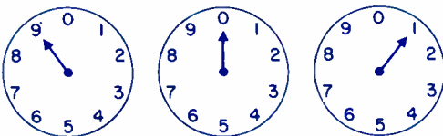
FIG. 1. A watt-hour meter in the decimal numbering system.
