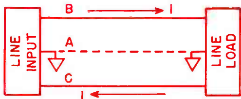
FIG. 2. Balanced line operation.
