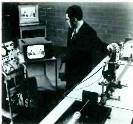
Courtesy General Telephone & Electronics Corp. FIG. 10. A laboratory model of a communications system which transmits and receives television pictures on a light beam generated by a laser.
