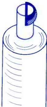
FIG. 2. AC relay magnet showing heavy metal "D" shaped band on one pole end.
