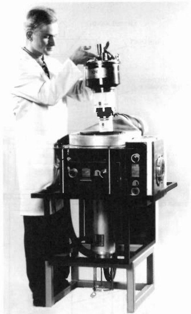
Figure 5. Manual installation of IOT7320R into operating circuit IM7320R
