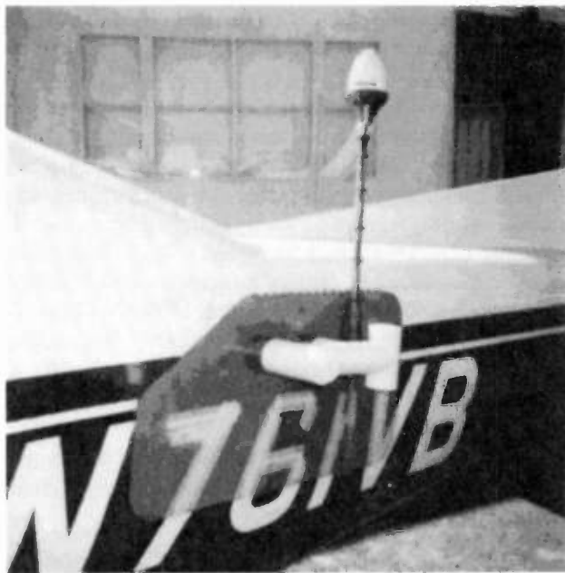
Figure 2. Medium-wave measurement antenna.
