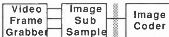
Figure 1. First-generation hardware architecture. The frame grabber output in first-generation systems is typically five bits for each of R,G and B. After image subsampling, the 128x96, 16-bit image represents a data rate of just 700K bytes/second. This data stream can be sent across a bus to a second board for further compression.
