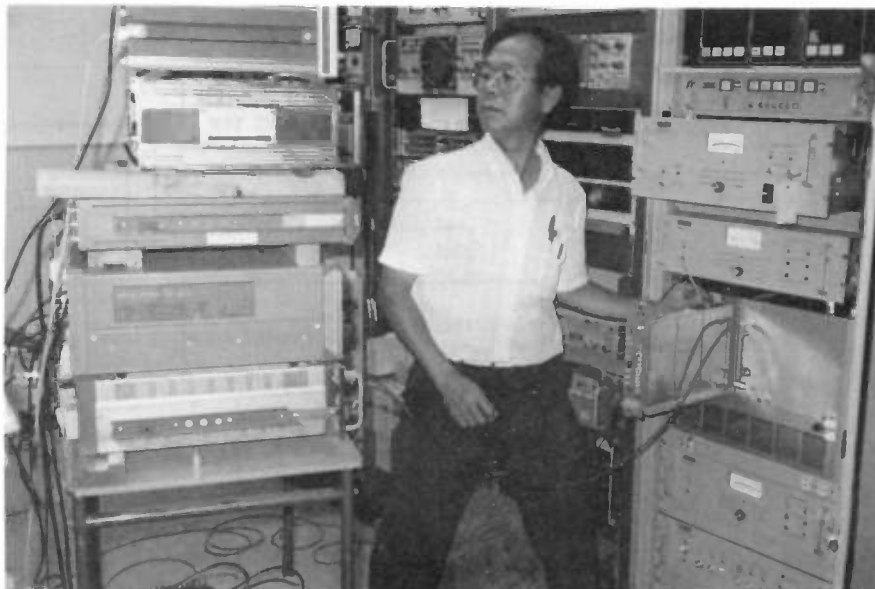
Figure 4 - Modulator Linearity Correction System under adjustment (Wrens, Georgia)
