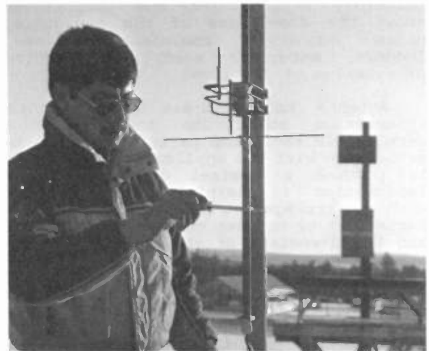
Figure 9 - Reduced-scale model antenna on manufacturer's test range. (courtesy Shiveley Labs)
