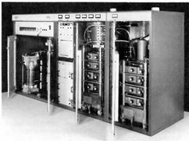
FIGURE 9. 60 kW TRANSMITTER WITH MSDC VISUAL KLYSTRON
