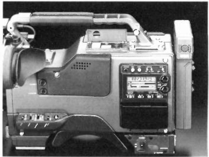
FIGURE 19. BVW-200 PHOTOGRAPH. SHOWING PRIMARY OPERATIONAL CONTROLS AND DISPLAY.
