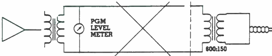
Fig. 1. DON'T meter the signal across the input to the repeat coil (transformer at rt.) and DON'T feed the repeat coil directly from another transformer, if possible.
