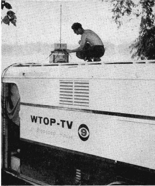
FIG. 5-21. 35-watt 26-Mc FM transmitter-receiver temporarily installed on mobile-unit roof for communicating with boats during Jimmy Dean Water Thrill Show on Potomac River. "Walkie-talkies" transceivers (see Fig. 5-22) were used in a boat towing Dean on water skis as well as in the amphibious "Duck" (see Fig. 5-18c). Contact with WTOP-TV master control was also possible (see Figs. 5-20a and b).
