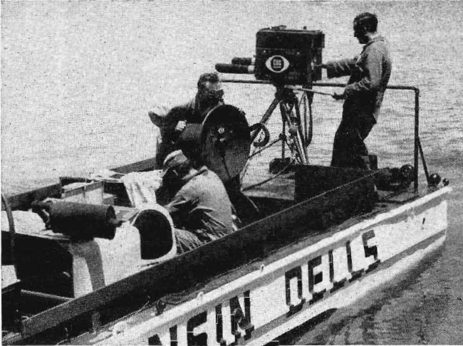
FIG. 5-18b. Close-up view of gasoline motor-generator (left), camera control unit, microwave transmitter, and camera installed in amphibious "Duck" for Jimmy Dean Water Show. Note 2-ft reflector used on microwave transmitter.
