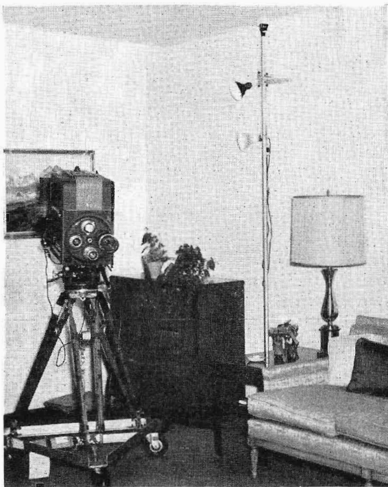
FIG. 5-26. Vertical "polecat" consists of telescoping spring-loaded aluminum tubing. "Clip-on" lights are shown attached to polecat.
