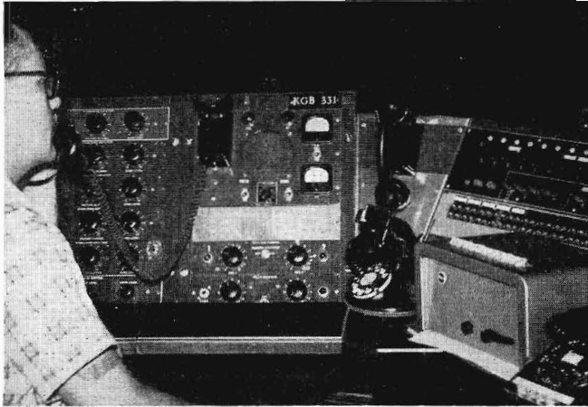
FIG. 5-20a. The control equipment for the 50-watt 26-Mc radio communications transmitter-receiver is operated from TV master control desk. This equipment is used for communications with the TV mobile unit.
