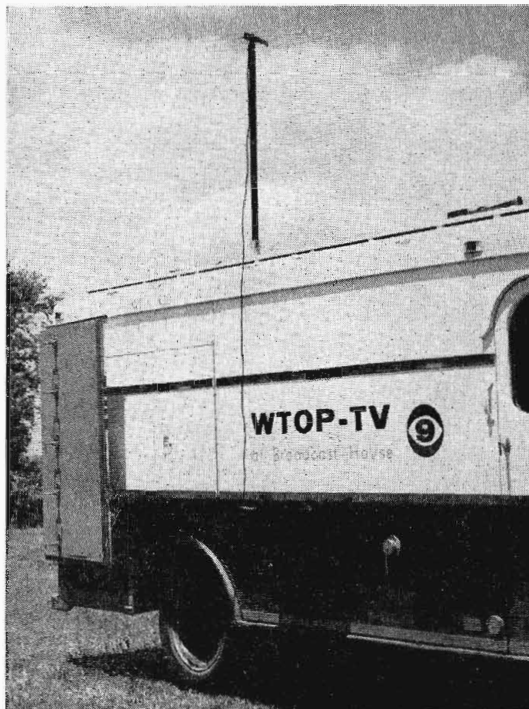
FIG. 5-4. Access to roof of mobile unit is by means of built-in steps on rear door. Detachable mast is used to support off-the-air receiver antenna as well as camera and microphone cables when required to bridge sidewalks.
