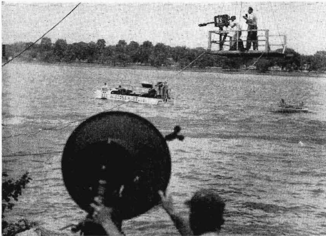
FIG. 5-18a. 2-ft microwave reflectors are used on the receiver (above foreground) and on the microwave transmitter in the "Duck" because of the broader microwave beamwidths as compared with the more common 4-ft reflectors. Note aiming sight attached to rim of reflector.
