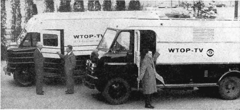
FIG. 5-1. RCA type TJ-53A mobile unit (foreground) designed for three-camera monochrome operation. This particular mobile unit was modified by WTOP-TV to accommodate four cameras. An older RCA model TJ-50A mobile unit is also shown.
