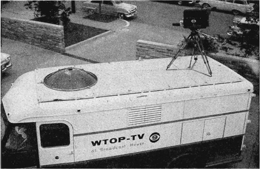
FIG. 5-3. Microwave reflector storage is shown on the left. On the right a camera is secured to the mobile-unit roof by use of a metal T and a chain from the tripod to a hook welded to metal roof.
