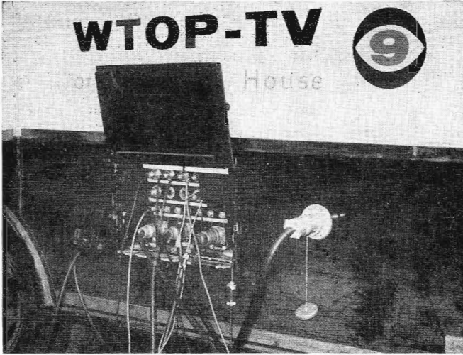
FIG. 5-11. 70-amp two-conductor rubber-covered power cable and connector are shown at right. Audio-video patch panel (left) provides rapid and convenient connection between mobile unit and cameras, microphones, telephone lines, microwave, etc.
