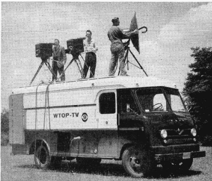
FIG. 5-2. The television mobile unit should provide a sturdy roof platform capable of supporting cameras, microwave transmitter, and operators.
