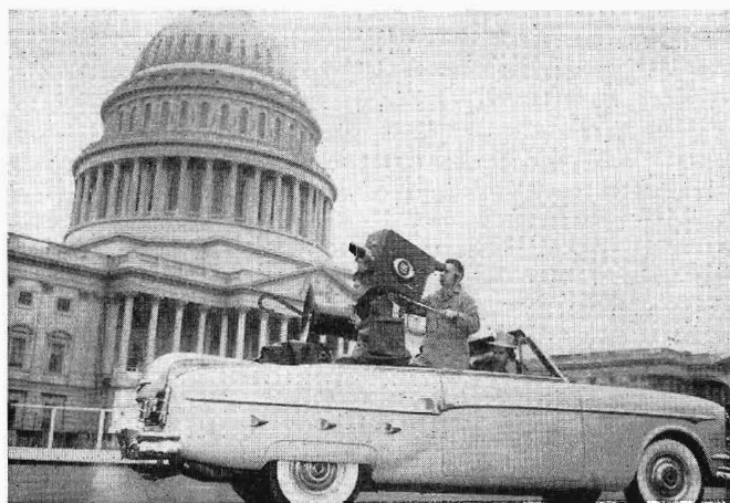
FIG. 5-18e. This Packard convertible was used during the inaugural parade in January, 1953, to relay continuous close-up pictures of President Eisenhower to a microwave receiving point on the roof of the U.S. Capitol. Not visible is the 3-hp gasoline motor-generator installed in the trunk. Accurate panning of microwave reflectors is required to prevent loss of picture signals.
