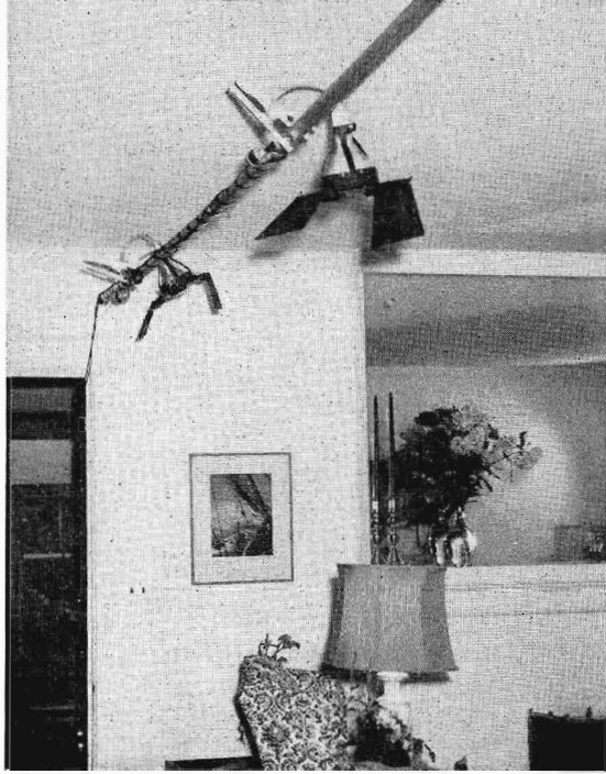
FIG. 5-27. Horizontally mounted polecat showing two "clip-on" light fixtures with barn doors for preventing direct light from falling into camera lenses.
