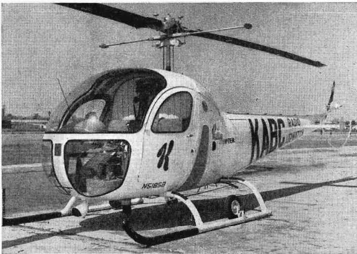
FIG. 3-7. Over-all view of helicopter showing 26 Mc antenna.
