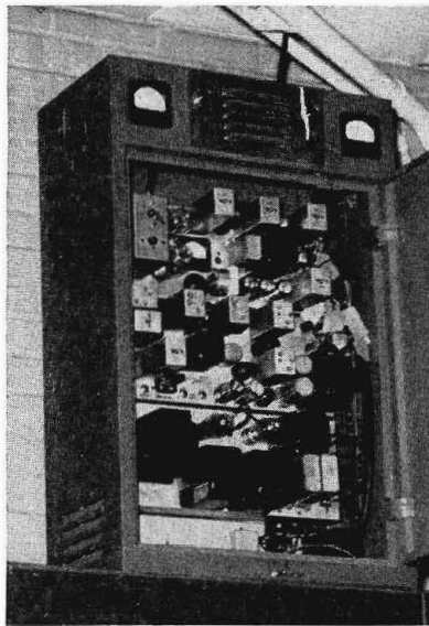
FIG. 5-20b. 50-watt 26-Mc FM transmitter-receiver operated from WTOP-TV master control.
