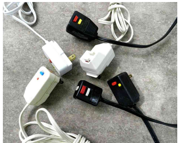
ALCI plug and cord sets removed from used hair appliances found in flea markets and thrift stores. All have the two buttons for “Test” and “Reset”.
