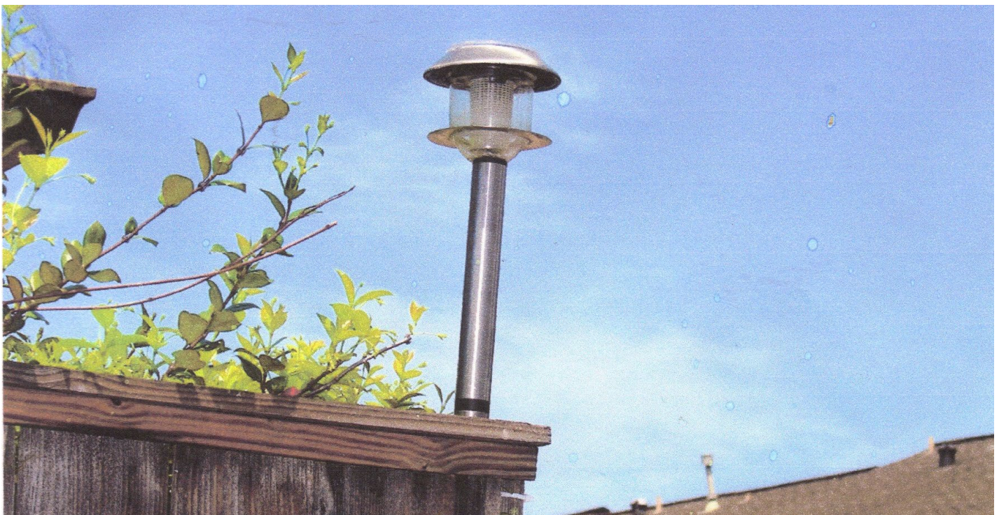
Bill Bowers' photo of his rooftop stealth antenna. (Courtesy: Bill Bowers)
