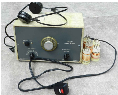
Knight “Ocean Hopper” retrofitted with an ALCI plug and cord for safety.
