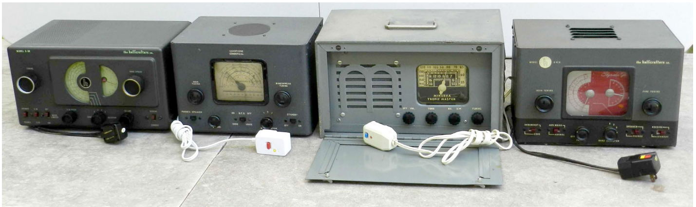
Metal radios retrofitted with ALCI plugs. Left to right Hallicrafters S-38, Echophone EC-1, Minerva Tropic Master and Hallicrafters S-41.
