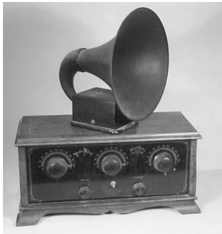
The three-dialer's five tubes provided decent sensitivity and selectivity as well as power to drive the horn speakers of the era.
