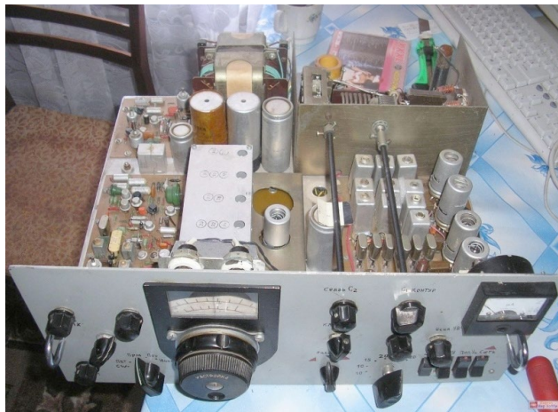
From the 1970s through the 90s, countless thousands of 80-10 meter SSB/CW transceivers just like this one were home-built by Russian and Eastern European hams. (Photo and info courtesy of Andrew Fedorov, KL1A, RW3AH [and about 30 other call signs!], creator of www.cqdx.ru , affectionately known as "Sparky," and presently based in Bonn, Germany.)
